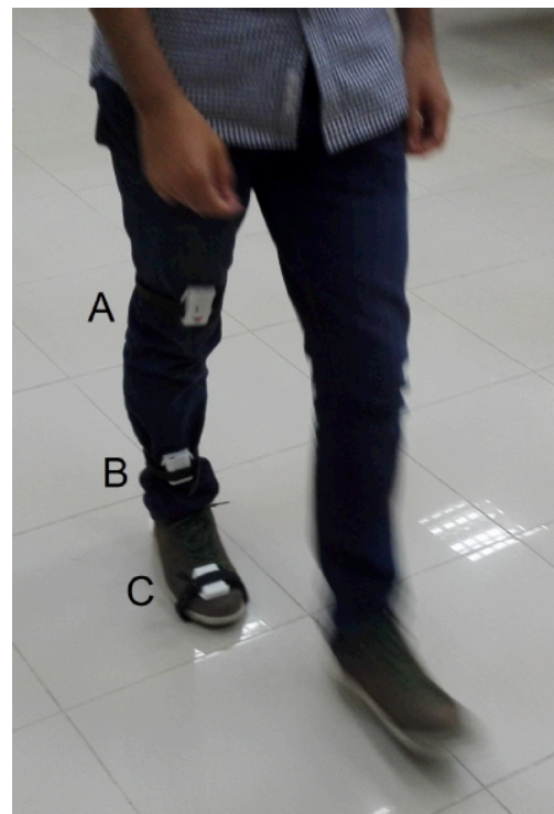
Figure 5. Location of sensors for measurements, A: Hip sensor, B: Knee sensor, C: Ankle sensor
