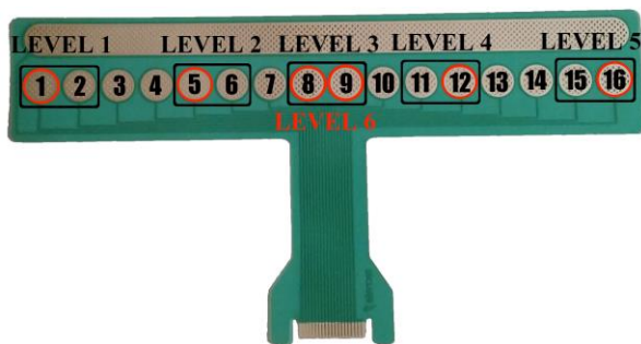
Figure 2. The stimulation array electrode, consists of 16 circular cathodes and a single anode stretching alongside, used for electrotactile feedback. The pads used for feedback mapping are marked with black rectangles (Levels 1 – 5) and red circles (Level 6).
